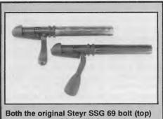
and that of the SSG-PIIK (bottom) are identical except that the SSG 69 bolt had a so-called "butterknife" bolt handle while those of the Police series have large knob-type bolt handles.
